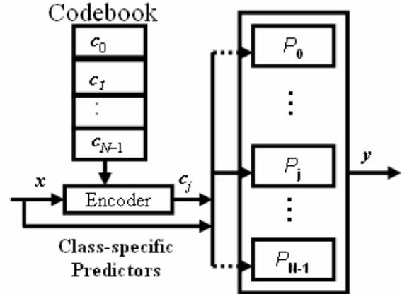
**Figure 1** A block diagram of our example-based image super-resolution algorithm, which is composed of a content-based encoder in the form of a vector quantizer, and a group of class-specific predictors to infer the high-frequency details.
