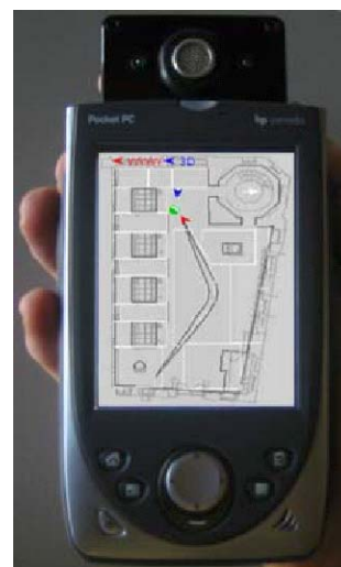
Figure 6 2D raster map displayed on a HP Jornada 568 handheld PC. The three cursors at the top of the figure represent the three users.
