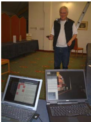
Figure 1 Early prototype of the system showing the web user view (Dub) on the left-hand machine, a desktop version of the VR user view (Ana) on the right-hand machine and a user carrying the PDA (Vee).
